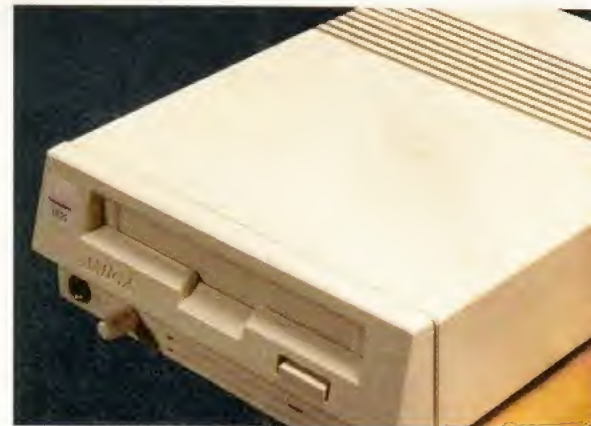
The A570 is useful for A500 users to upgrade to CD-ROM, but doesn't have a standard SCSI interface.
